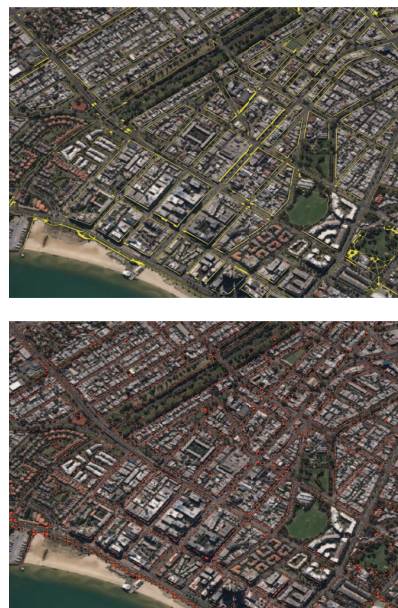
Fig. 1. An example of the ground truth footpath network in an area of Melbourne. The figure on the top is the ground truth footpath network and the figure on the bottom is generated by our pipeline automatically. The background map is provided by Bing Aerial.
