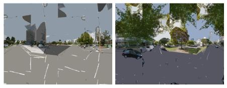
Approach based on mean shift (Comaniciu and Meer, 2002). Panels arranged to allow sky colors to flow together. Utilize which colors are above and below image center. Preprocessing step to analyse sky colors and amounts to pick mean shift parameters.
