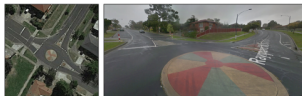
(a) Compact roundabout with stop line and ending bicycle lane (region B)
