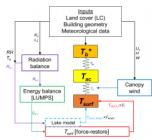
The Air-temperature Response to Green/blue-infrastructure Evaluation Tool (TARGET) is a computationally efficient model designed to evaluate blue/green infrastructure, based on an urban canyon and aggregations of different land cover types [Broadbent et al., 2019].
