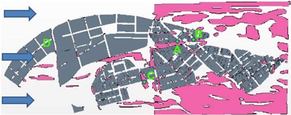
**Figure 22 10 m/s exceedance plots for wind from West at z = 2 m (ground level) (green text shows case study areas described in more detail below, red circles indicate high winds in public spaces)**
