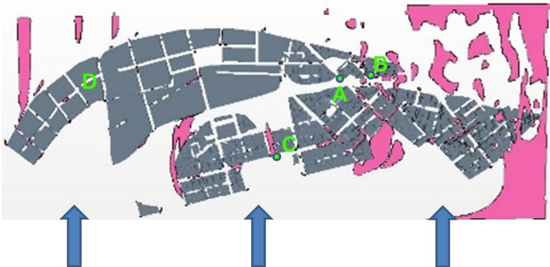
**Figure 21 10 m/s exceedance plots for wind from South at z = 2 m (ground level) (green text shows case study areas described in more detail below, red circles indicate high winds in public spaces)**
