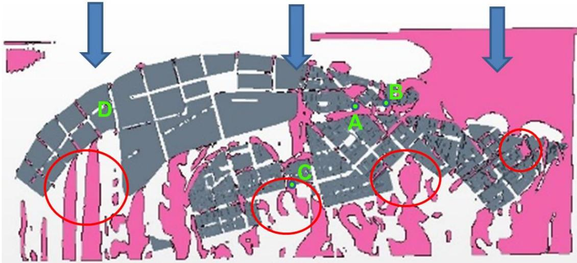
**Figure 20 10 m/s exceedance plots for wind from North at z = 2 m (ground level) (green text shows case study areas described in more detail below, red circles indicate high winds in public spaces)**
