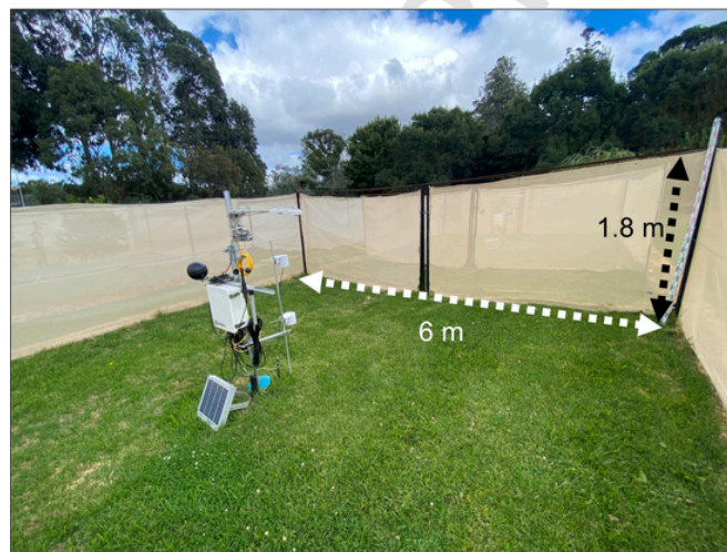
Fig. 1. Six identical plots (6 × 6 m) were set up at the Burnley Campus of the University of Melbourne. Three were unirrigated and three received 4 mm of irrigation at 13:00 every day. Each plot was surrounded by 1.8-m tall 70% shade cloth (SOLARSHADE™) and a climate station was installed at the centre of each plot to continuously monitor the microclimate, soil temperature and soil moisture content.
