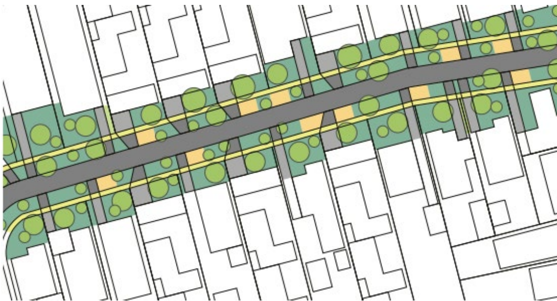
Figure 9. Example of water sensitive streetscape design. As found by (Meng and Kenway 2018) road design can have significant impact on overall precinct water performance. (London et al. 2020b, p. 44.)
